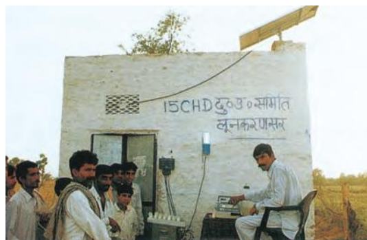
Fig. 5.11: Solar operated electronic milk testing equipment
