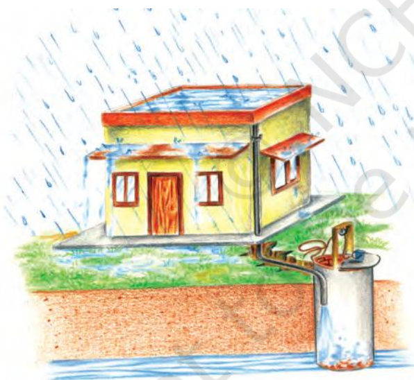
(b) Recharge through Abandoned Dugwell
