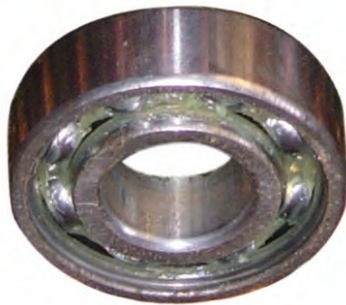
Fig. 12.16 : Ball bearings reduce friction
