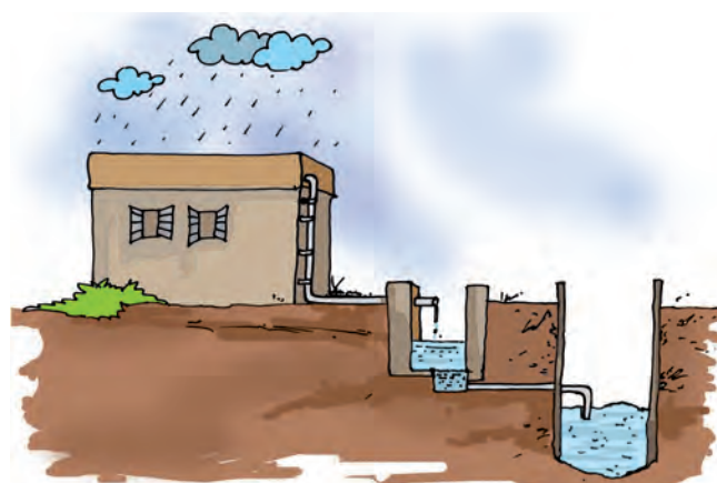
Fig. 14.13 Rooftop rainwater harvesting
