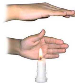
Fig. 4.10 Transfer of heat by convection in air
