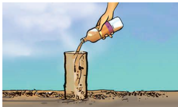
Fig. 9.5 Measuring rate of percolation
